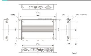
\*1 When you fasten the bundled attachment fittings to be fixed to the body, you should use the attached screws  $(M3 \times 6)$ . Otherwise, the length (L) from the surface of the cabinet to the screw tip should be 4mm or less.
