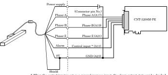
\* When the control input is set as a general-purpose input, the alarm output state can be checked When the control input is set as the counter stop input, the counter can be stopped at alarm output.
