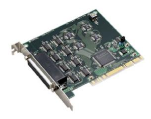
This board is a PCI bus interface board for performing RS-232C serial communications with external devices.
