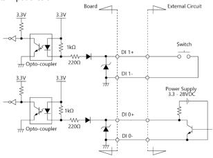
The signal input is a non-isolated opto-coupler input (with current sink output support). A current of 6.4mA is required to turn the input on, and a leakage current of 0.16mA or less is required to turn the input off.
