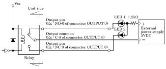
As a result, setting output NO-0 to "ON" state (make status), LED1 comes on and LED2 goes out.
