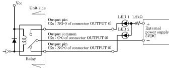
As a result, setting output NC-0 to "ON" state (make status), LED1 goes out and LED2 comes on.
